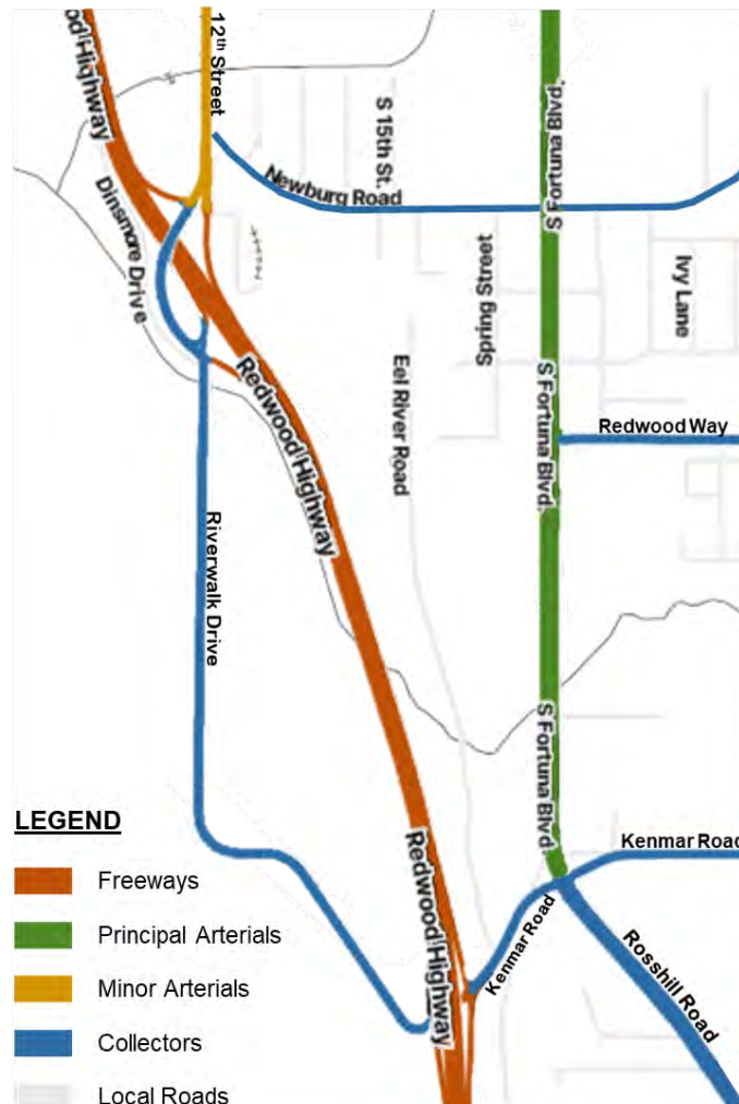
Figure 2 Existing Road Facilities
